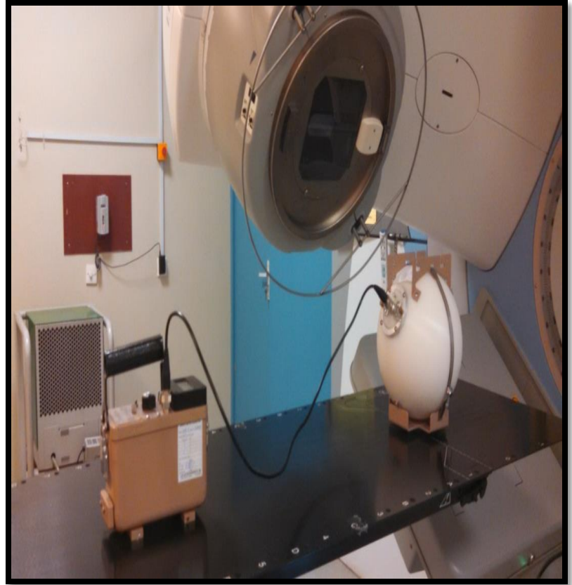
Fig. 2: Setup for Measurement of Neutron Contamination in 3D CRT AND ssIMRT
